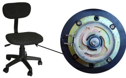
Figure 1: Vibration motor mounted beneath the seat of an office chair.
