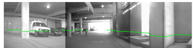
Figure 4. 180 Degree FOV image provides a human friendly interpretation to the LIDAR data processed by the vehicle.
