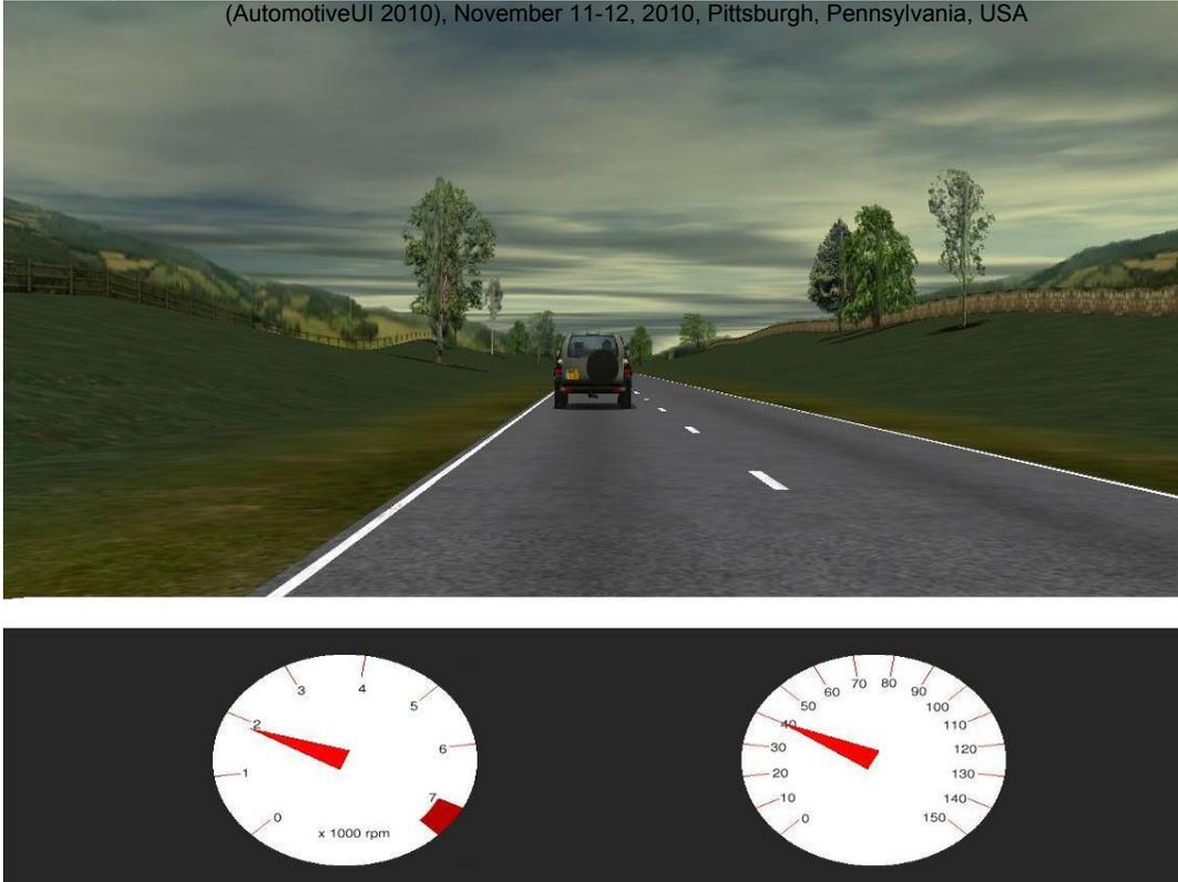
**Figure 2 – The simulated driving environment including road scene with lead vehicle and in-vehicle dashboard**
