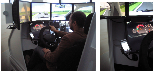
Fig. 1. Left: The driving simulator used in the evaluation. Right: Detail, showing the placement of the mobile phone running the speech interface.
