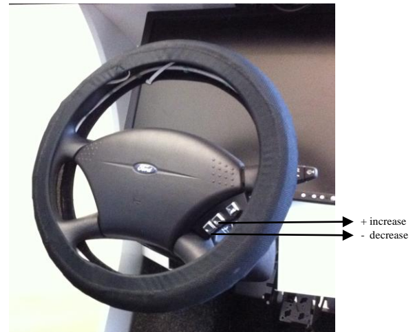
Figure2. Push-button interface built on the steering wheel.
