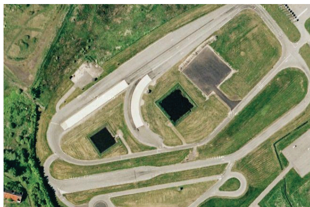
Figure 3. The driving circuit used in the experiment. The two white sections in the middle, left of the picture are the slippery road sections.
