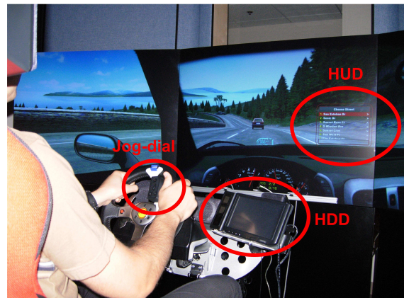
Figure 1. Driving simulator with head-up (HUD) and head-down (HDD) screen positions indicated. A jog dial controller is mounted to the steering wheel.
