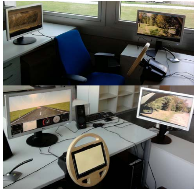
Figure 1: Prototypical implementation of our multimodal interaction style – a microphone captures speech commands while gestures are performed on a multi-touch steering wheel. Screens around the driver's seat simulate the back window, driver/passenger windows and the exterior mirrors. The front screen displays the driving simulator and a virtual dashboard.
