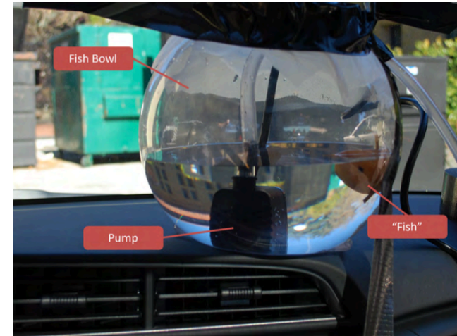
Figure 1 - Fish bowl prototype to provide visual feedback on driving behavior.
