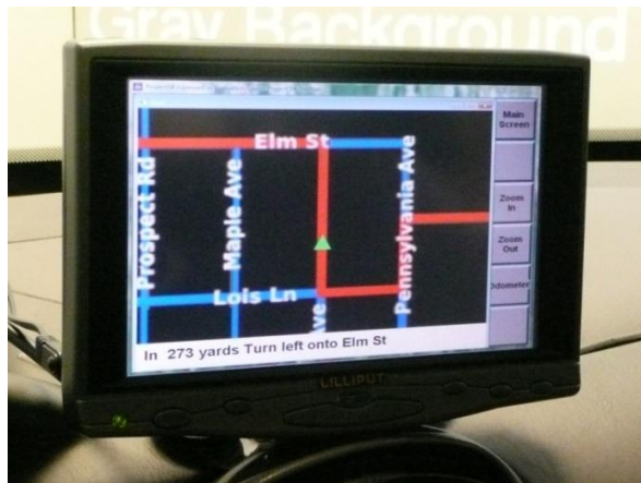
Figure 3. LCD screen displaying real-time location of the vehicle on a map.
