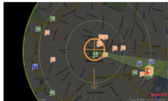
Figure 4: Overlay (orange cross and arrow) which indicates the direction to the next task and selectable POI to participants.
