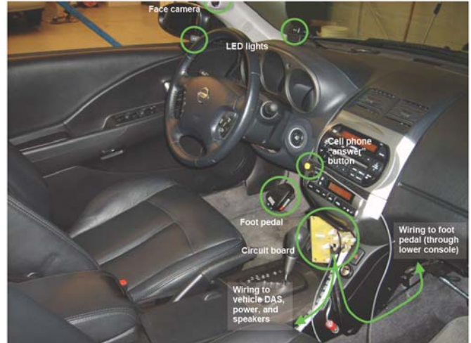
Figure 2. Layout of the instrumented vehicle for on-road testing.
