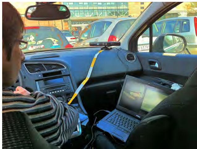
Figure 1 - Reference configuration for a Kinect in a car
