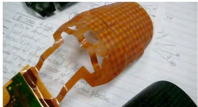
Figure 5. Capacitive film from off-the-shelf mouse
