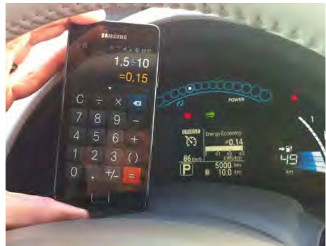
Figure 1. An experience EV driver demonstrate how he calculates the required energy efficiency for traveling 10 km using 1 battery bar (1,5 kWh) in a Nissan Leaf.
