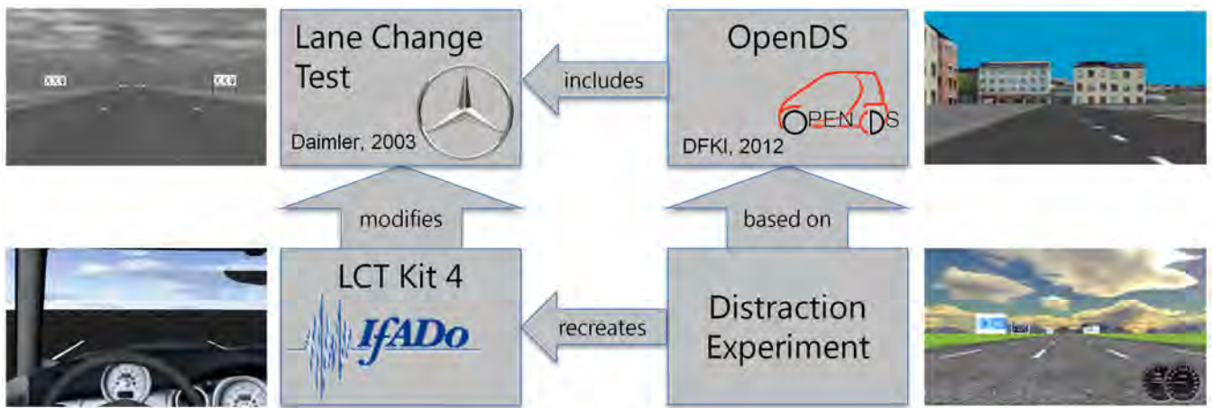
Figure 1: The distraction experiment described here is a reimplemention of the LCT Kit in our OpenDS driving simulator. It is based on the Lane Change Test, but measures reaction time instead of lane deviation.
