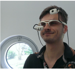
Figure 1: In this image, an gaze-tracker is constructed by combining two lightweight cameras: (1) a camera under the eye that tracks the pupil, (2) a camera that captures the user's viewing frustum. Photo: Courtesy of Valentin Schwind, University of Stuttgart.
