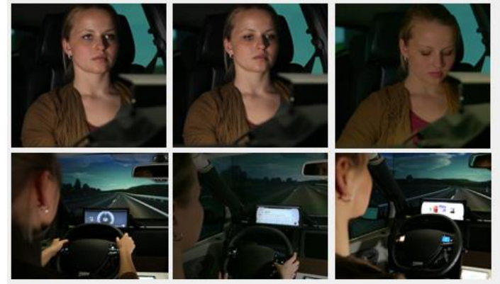
Figure 1. The position of the head and hands for each condition. From left to Right: SAE Level 2 Baseline with hands on wheel, SAE Level 3 Mobius and SAE Level 3 Smartphone.
