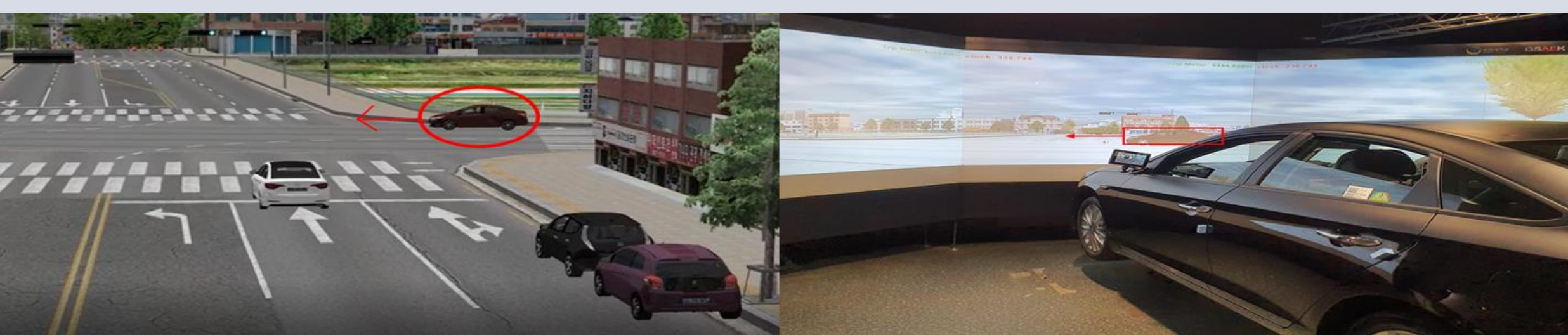
Figure 1. Scenario (left) and driving simulator for data acquisition (right)
