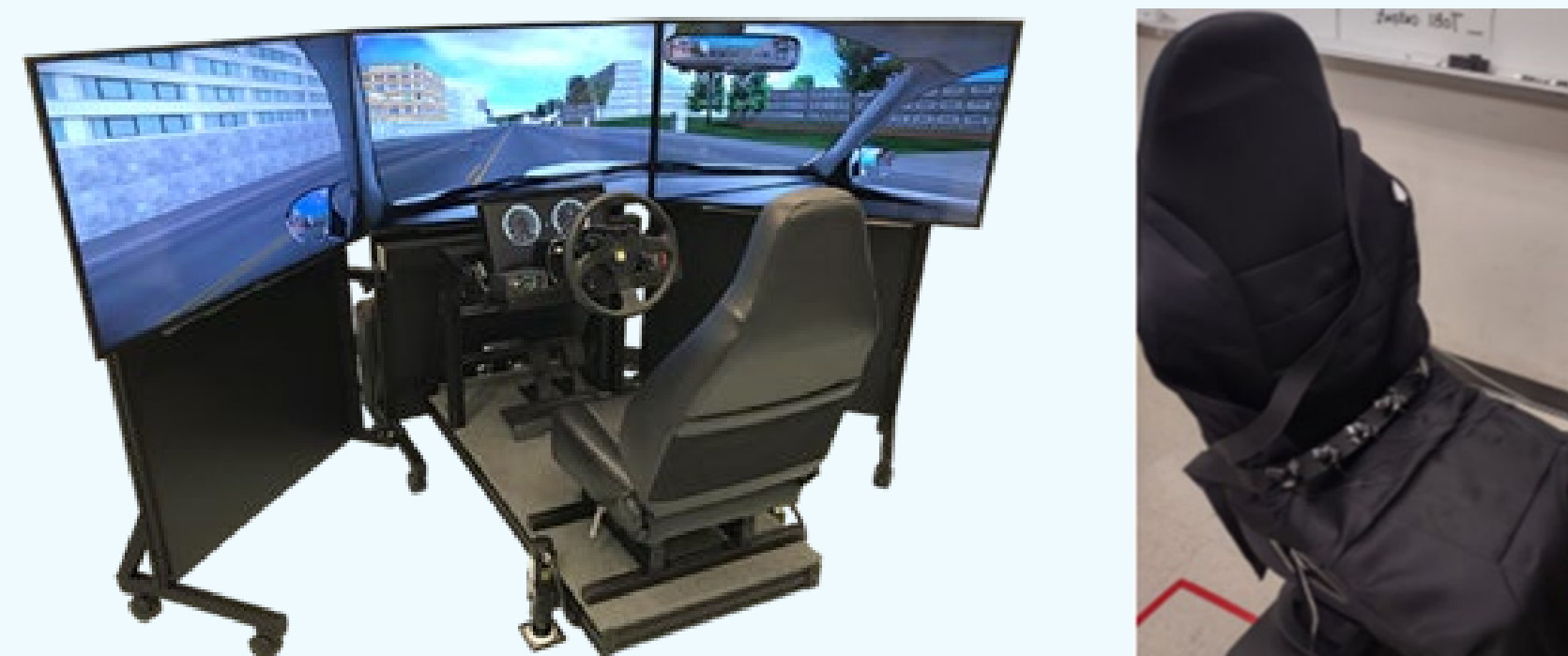
Figure 2: MiniSim Driving Simulator and Tactile Seat and Seat Belt
