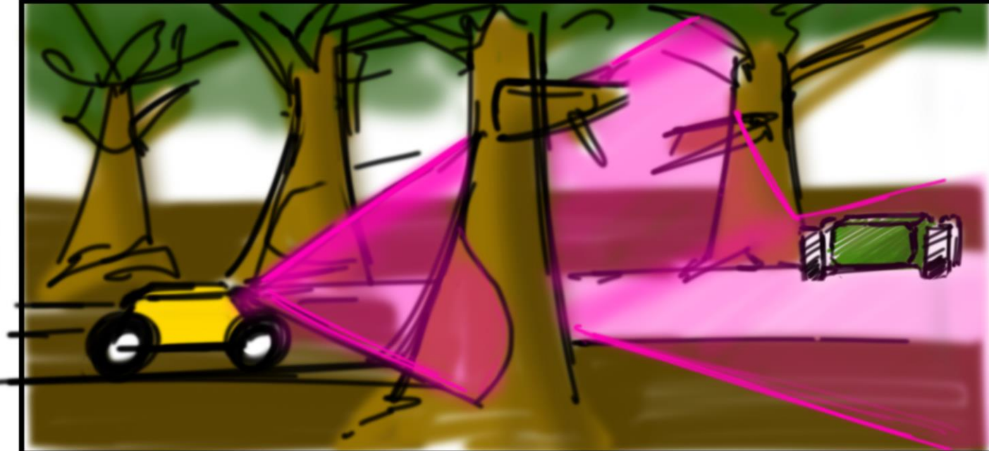
Figure 1: Storyboarding the interaction concept: a remote reconnaissance vehicle follows a set path, its sensors register an unknown object, which can then be classified by the operator.
